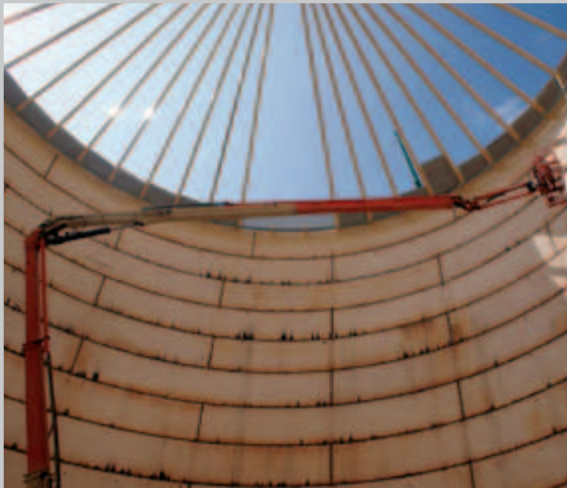
Unmatched range of motion. With Up and Over height of more than 18m and 19m of horizontal outreach, the 1250AJP gets you where you need to work.
