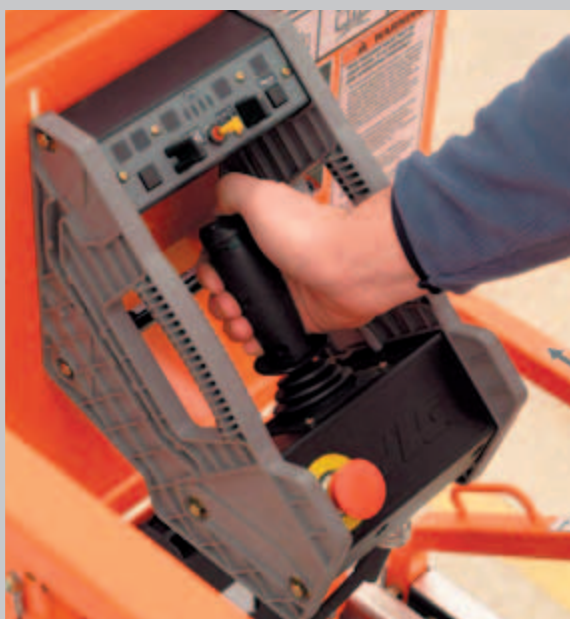
Fully proportional control of drive, and lift functions
