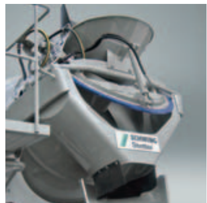
3/4-flap – Drum cover It prevents liquid contents from spilling when the truck is started, braked or driven uphill.
