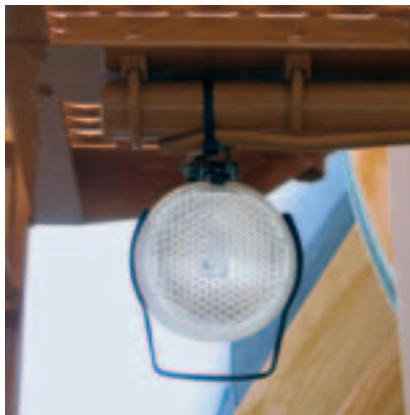
Working searchlight Mounted below the ladder platform to illuminate the unloading area.
