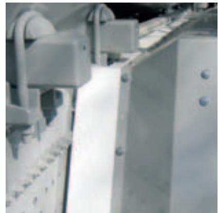
Widening of mudguards Protects the truck mixer from severe soiling on and off the road. Recommended in conjunction with the frame covering.
