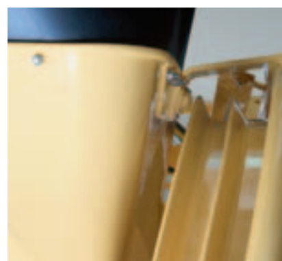
Double dripping ring: even less soiling in the discharge trestle area
