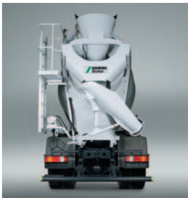
The 1,450 mm long swivel chute facilitates discharge into the concrete pump hopper.
