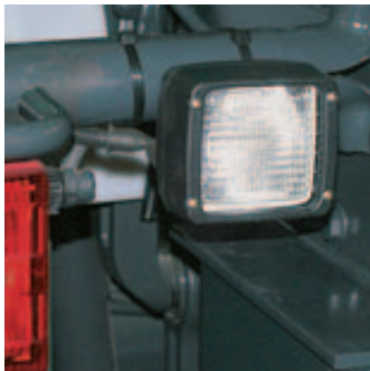
Halogen floodlight At the rear of the machine for illuminating the unloading area.
