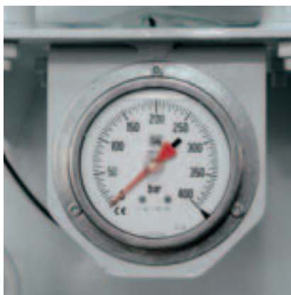
Slump meter The pressure gauge shows the operating pressure of the hydraulic system and gives a reference value for the change in concrete consistency with unchanged loads.
