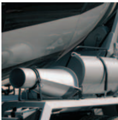
Adapter piece: Flow concrete pipe The adapter piece enables connection of additional delivery pipes for the pouring of flow concrete.
