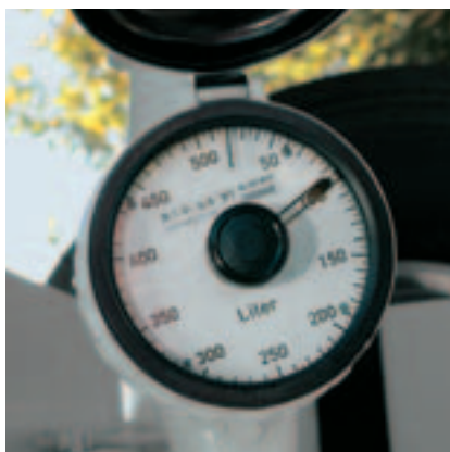
Water meter With scales for 500 or 1,000 litres for precise proportioning of water.
