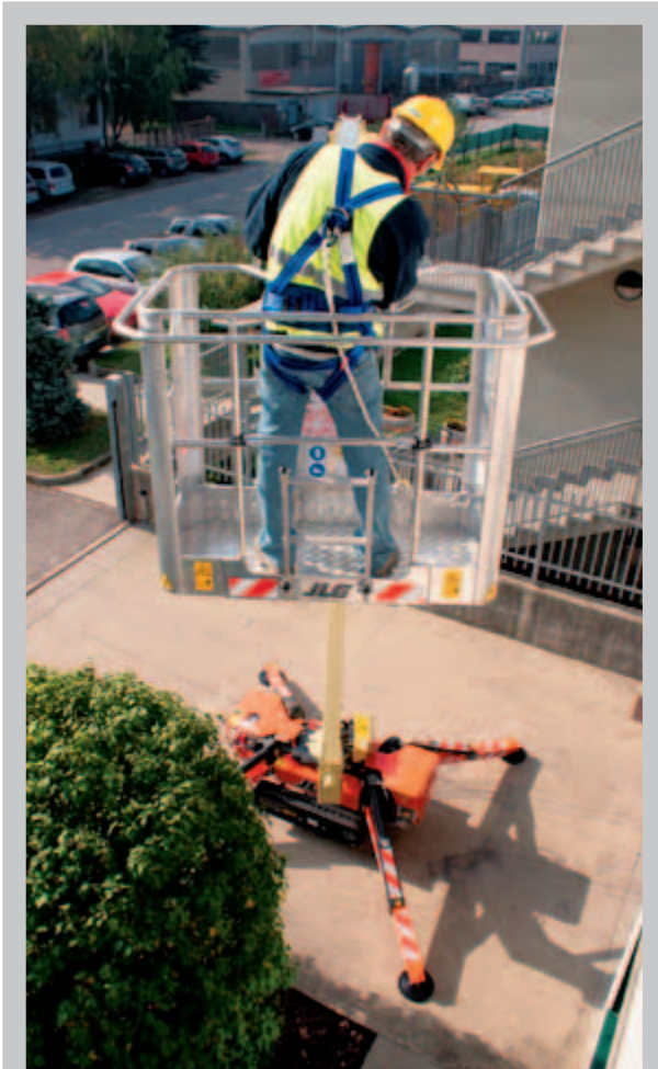
Square outrigger pattern for additional stability
